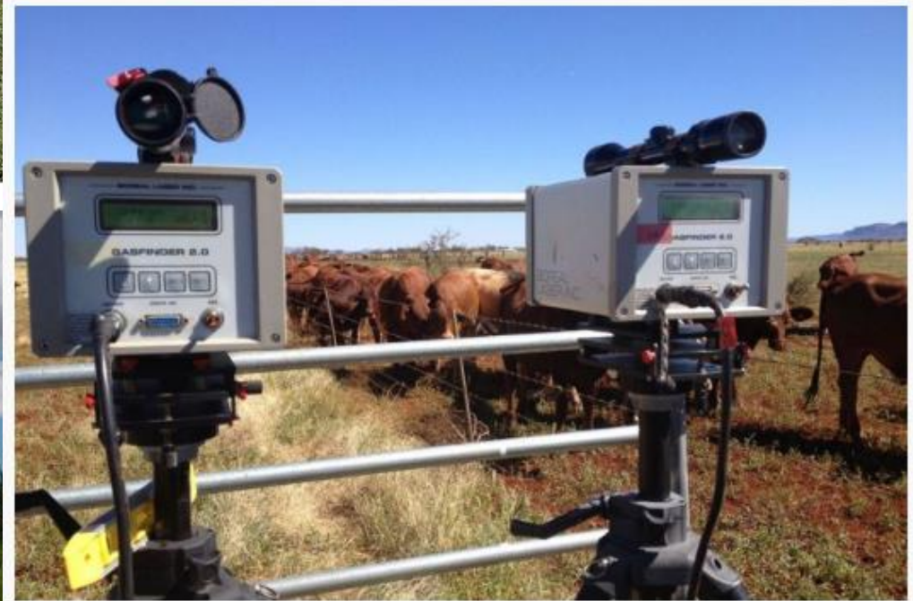
PHOTO: Rob Kinley said in previous projects they have used open path lasers to measure methane in the field. (Supplied: Rob Kinley )
